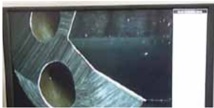
A high resolution image of a re-sharpened gun drill
