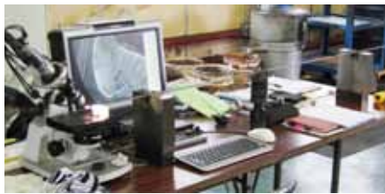
Inspection of a 2.8m long gun drill using a tillable vision system
