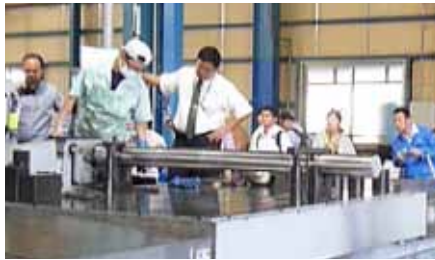
A 2.0m 2 Column Type Gun Drill Machine with an Incoloy 718 Benchmark Test Piece
