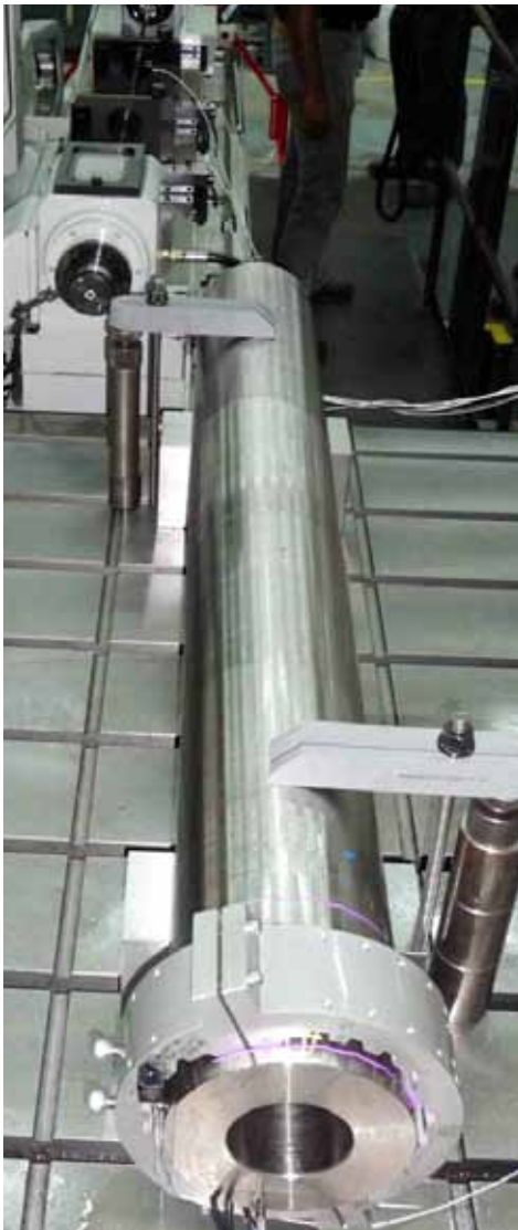
1.6m work-piece set up with Advanced Sensory System for Drill Slippage Detection
